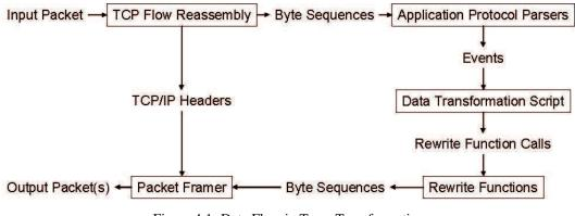
Figure 4.1: Data Flow in Trace Transformation
