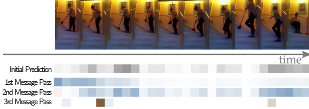
Figure 4. Evolution of prediction with increasing messages passes. The first row shows the initial prediction for the category tidying with a broom without any message passing, where darker colors correspond to higher likelihood, blue is then an increase in likelihood, and brown decrease. In the first message pass, the confidence of high predictions gets spread around, and eventually increases the confidence of the whole prediction.
