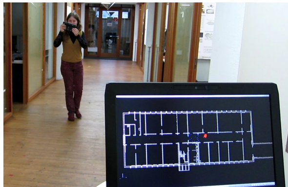
Fig. 1. Localization in 6DoF using only a 2D outline of the environment and an RGB-D Google Tango device. The computer screen shows the floor plan in white and the particle cloud representing the current pose estimate in red.
