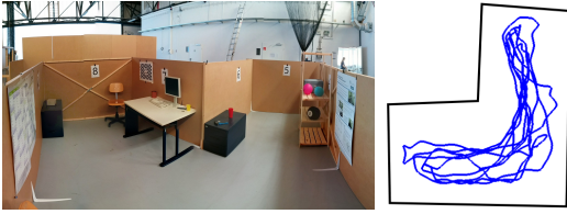
Fig. 3. For accurate metric evaluation, we built an L-shaped and furnished indoor environment in a motion capture hall. Left: a photo of the setup. Right: the corresponding floor plan with the walked ground truth trajectory in blue.
