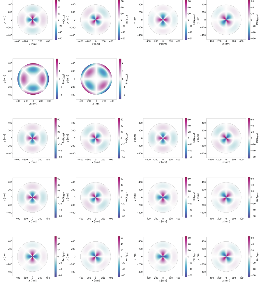
Figure 1: Real and imaginary parts of all components of the mode overlap integrand \mathcal{I}_{ijkl} for the LCP \rightarrow 3 \times LCP configuration (part 1).
