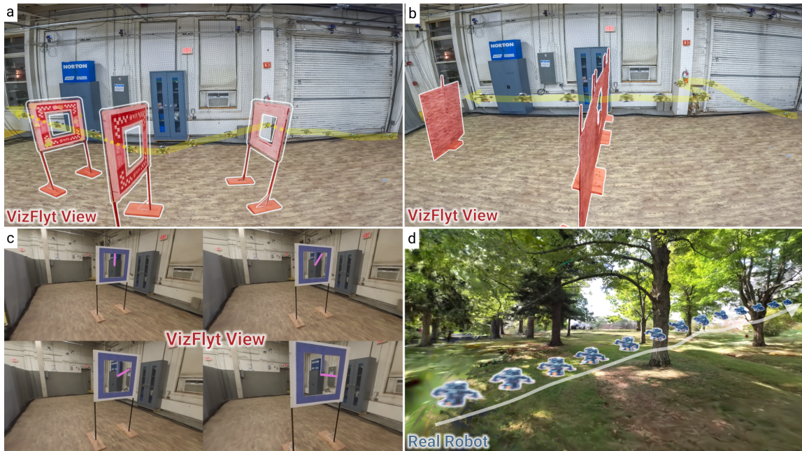
Fig. 4: (a) Flight test for proposed project 3: flight through racing windows, (b) Flight test for proposed project 4: flight through unknown gap, (c) Proposed project 5’s dynamic window and (d) High-speed flight experiment. The red highlights denoted as VizFlyt view show hallucinated cameras seen by the robot in (a) to (c). In (d), the entire scene is hallucinated with the real-robot overlaid.
