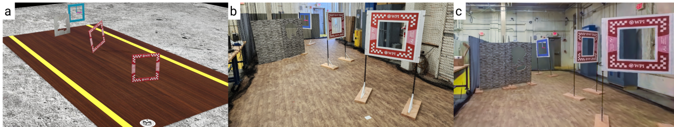
Fig. 1: Evolution of perception-centric offerings of the course. (a) course based on simulation, (b) course based on a real-world obstacle course, and (c) new course based on the proposed VizFlyt framework, where the image is a real-time photorealistic render of a hallucinated camera on an aerial robot used for autonomy tasks. All the images in this paper are best viewed in color on a computer screen at 200% zoom.
