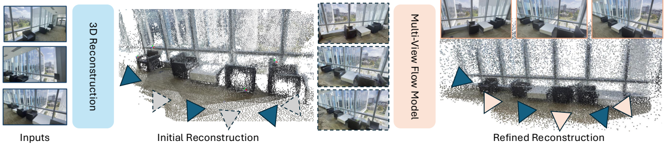
Figure 2. Overview. Given a set of source input images \mathcal{I}_{\text{src}} (blue), we use our robust reconstruction method (Section 3.1) to create an initial reconstruction result that can be rendered at various perspectives (gray). We use these renderings as the source samples of our flow matching model (Section 3.2), which maps the rendered images to the target distribution, i.e. ground-truth images. We use the generated views (orange) to improve the quality of the reconstruction (Section 3.3).
