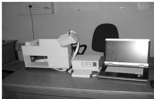
Figure 1. High precision real-time multichannel spectropolarimeter with binary polarization modulation
