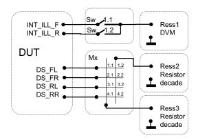
In our example there are three resources, one DVM and two resistor decades, that can be connected to the DUT. The DVM supports the method "get\_u", the resistor decades the method "put\_r". The following tables show the representation of this test circuit for the test stand:
