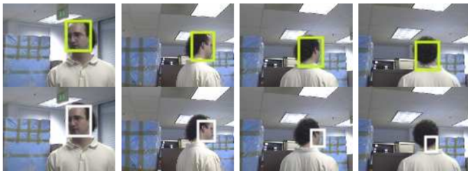
Fig. 11. Cubicle sequence 2. Tracking results of the proposed tracker (top) and particle filtering (bottom). Frames 9, 55, 60, 64 are shown. The video is of size 352 \times 288 and frame rate 30 FPS.
