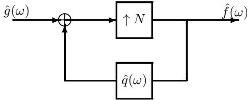
Figure 5: Block diagram of the FIF Generation.
