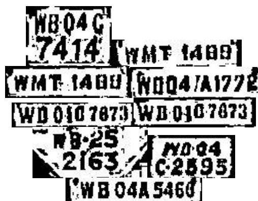
Fig. 5. Binarization result of our designed algorithm on the sample set of vehicle license plate images shown in Fig. 4.
