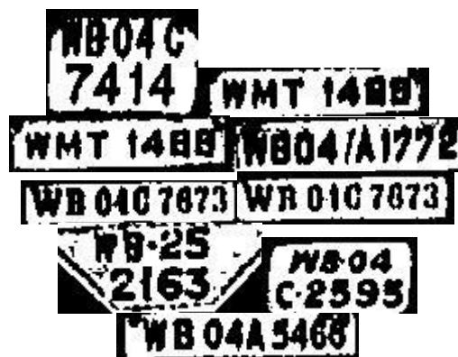
Fig. 6. Binarization result of Otsu's algorithm on the sample set of vehicle license plate images shown in Fig. 4.
