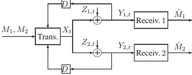
Fig. 1. The two-user Gaussian BC with noise-free feedback.
