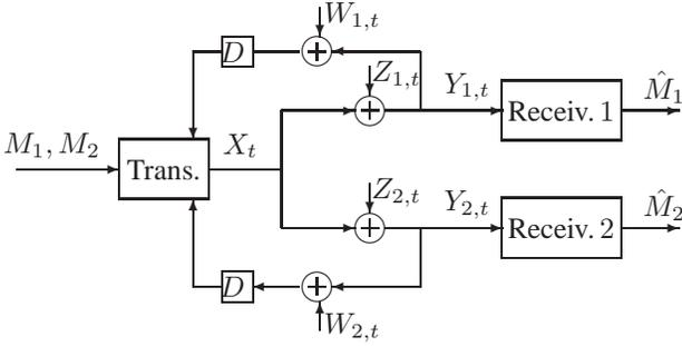
Fig. 2. The two-user Gaussian BC with noisy feedback.
