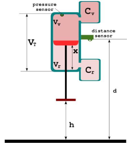
**Figure 5: Diagram of the setup.** Two chambers separated by the piston. Each chamber is connected to an additional chamber that does not change volume during the motion. The position of the sensors is also shown in the diagram.
