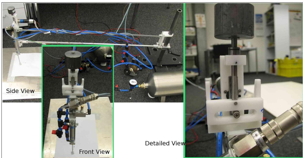
**Figure 4: Three views of Zürihopper.** The global view shows the complete setup. The way the mass is connected to the DC motor is observed in the detailed view.
