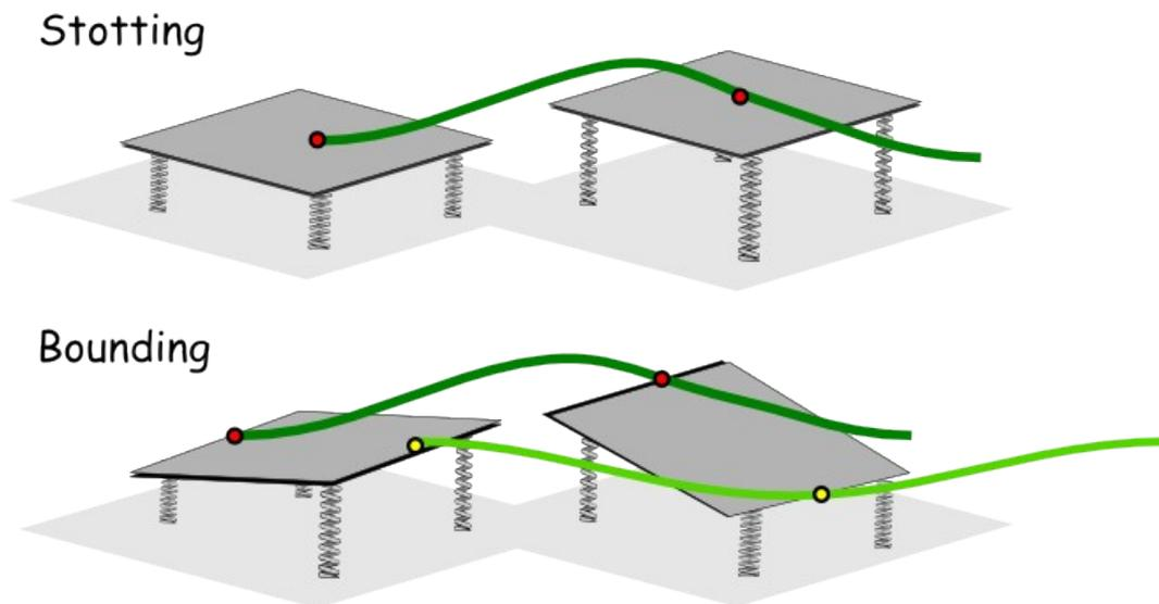
**Figure 18: Normal modes of a plate with springs.** Two possible normal modes resembling stotting and bounding gaits of quadrupeds. The lines depict the trajectory of the markers in the plate.
