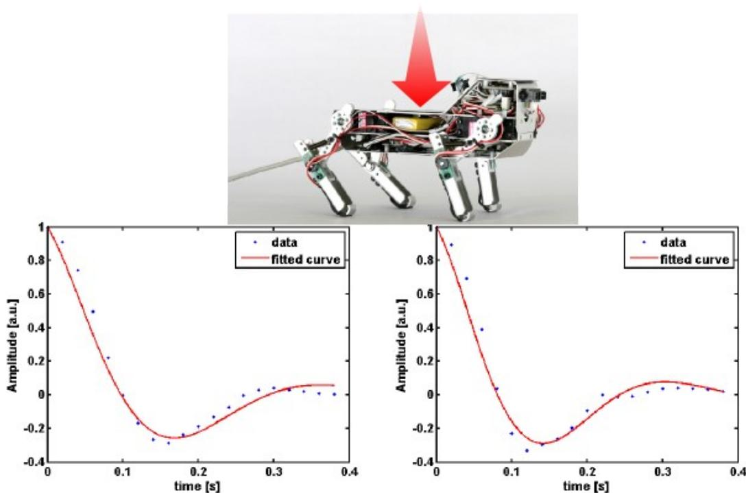
**Figure 19: Identification of Alan Puppy robot.** The step response of the legs of the robot are plotted. In solid line the best fit of a damper-spring system. It can be seen that the time scales of the responses differ; this can be associated with the effect of uneven mass distribution.
