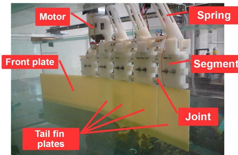
**Figure 13: The WandaX experimental robot platform** hanging from the frame and submerged around 4cm into the water. The most important parts are labeled with the terms used throughout the text.
