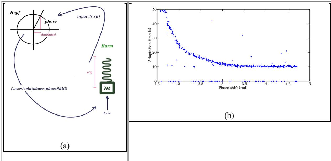
**Figure 15. Adaptive frequency Hopf oscillator coupled to a harmonic oscillator.** (a) Schematics of the setup. The Hopf oscillator acts as a controller and is sending a forcing signal to a simulated mass-spring harmonic oscillator. Its amplitude is then sent as input to the Hopf. (b) An experiment with phase lag introduced onto the feedback signal to the Hopf oscillator. This significantly affects the time of frequency adaptation.
