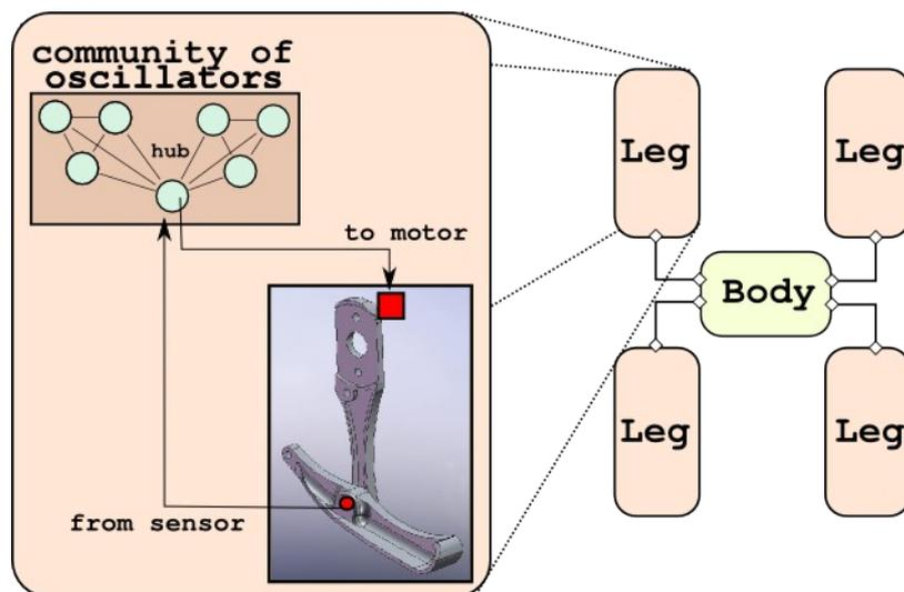
**Figure 16: Schematic of the proposed control architecture.** A CPG (central pattern generator) represented by a community of oscillators is influenced only by local information coming from the limb it controls. We are trying to determine whether this community can share information with the communities connected to the other limbs, through the environment and the body.
