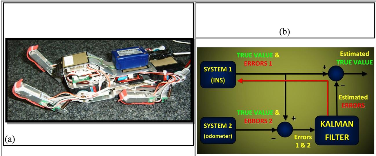
**Figure 20: Self-motion cue based navigation in the quadrupedal robot.** (a) Puppy II robot equipped with an additional Inertial Measurement Unit (blue box). (b) Fusion and error estimation algorithm. Information about the robot’s position, velocity and attitude is fused and errors are estimated and subtracted with a Kalman filter.
