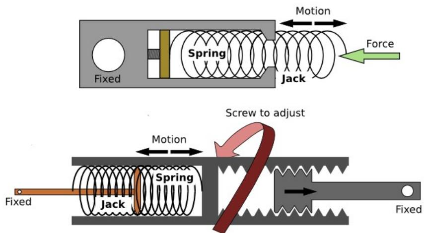
**Figure 3: Fix-length jack-spring.** This device is easier to mount than the usual design shown on top. It allows the installation of a motor to provide stiffness adjustment.
