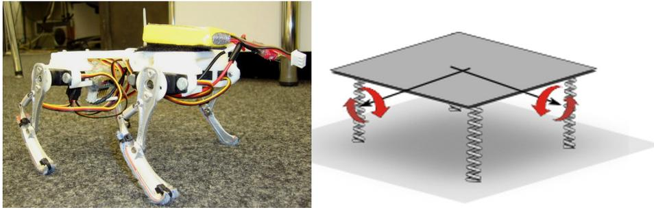
**Figure 17: Model of quadruped robot.** On the left a photo of the real robot. If we assume the legs are attached to the ground, it can be represented with the linear model shown on the right.
