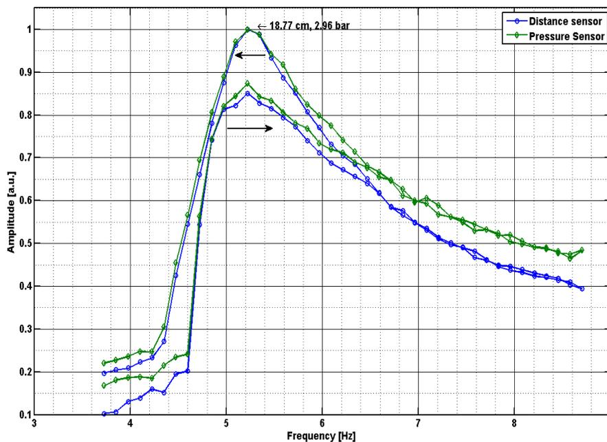
**Figure 8: Amplitude versus frequency.** There is a frequency for which the system shows maximum amplitude. Depending on how the frequency is varied, the value at which this maximum happens can change. The arrows indicate increasing and decreasing frequency.
