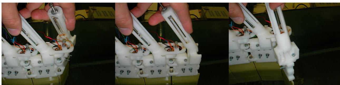
**Figure 14: Tunable spring in WandaX.** From left to right: the last segment is manually bent from the leftmost to center and rightmost position. The spring is extended more whenever the segment is not aligned with its neighboring one. The screw on top of the “spring tunnel” can be screwed in to shorten the spring. The force holding the segments aligned is then reduced and less force is needed for the same deflection.
