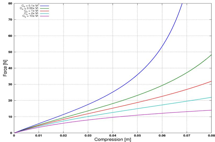
**Figure 6: Spring curves for different values of dead volume** connected to the upper chamber. This parameter changes the behavior of the spring from positive concavity to negative concavity.
