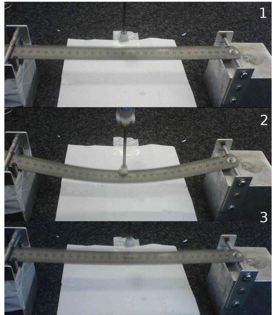
**Figure 7: Ground with variable stiffness.** This setup exploits the bending of a metal beam to produce stiffness depending on the length of the beam.
