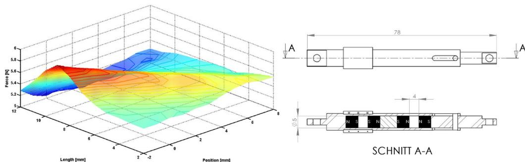
**Figure 1: Simulation of a magnetic spring.** On the left, force between the magnets at a nominal distance for different lengths and positions of the coil. Current at 400 mA. On the right, a schematic of the prototype. The fixed magnet lies inside the coil.
