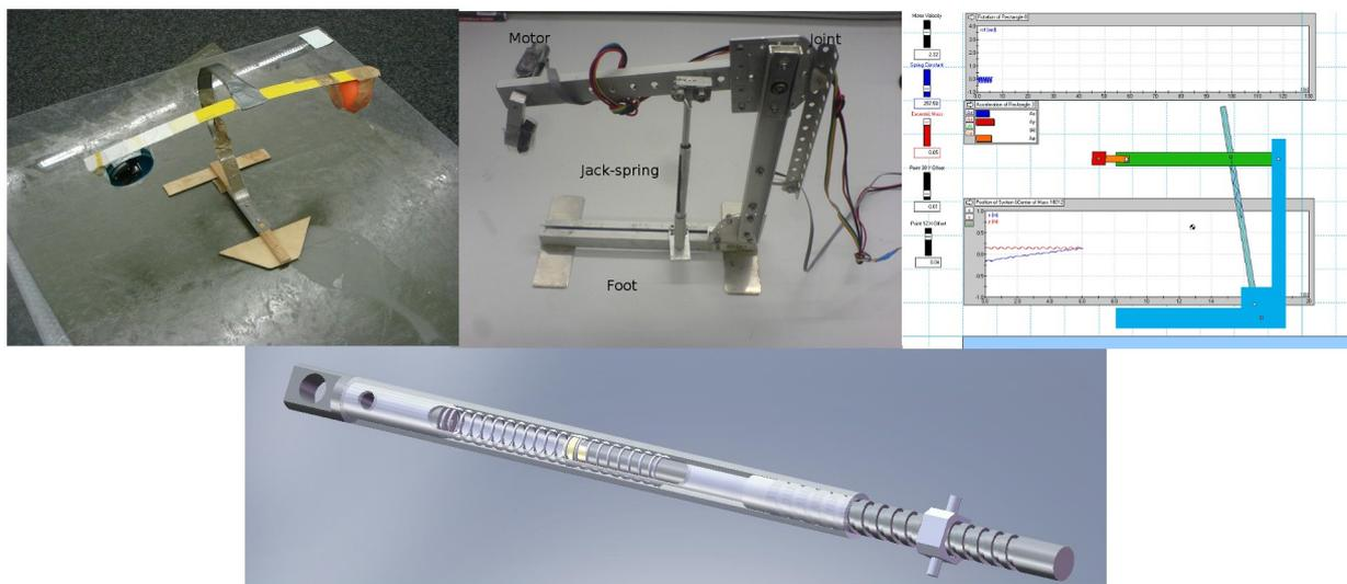
**Figure 11: Dumbo and its rigid counterpart.** On the top left a picture of Dumbo, to the right, Rumbo, the rigid version and a 2D model of it. On the bottom we show the CAD of the jack-spring.
