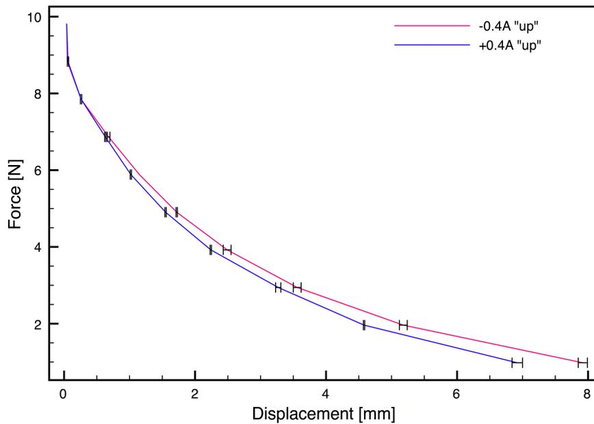
**Figure 2: Stiffness versus current.** Experimental results showing the change in the curve of the spring for two values of current (maximum ratings). The change in displacement is approximately 10%.
