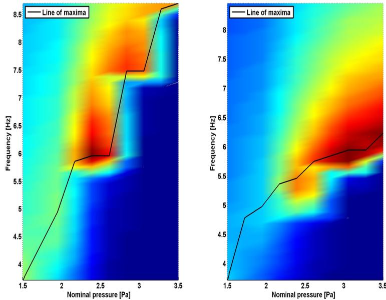
**Figure 9: Amplitude in the frequency-pressure plane.** The line of maxima is marked in black. A controller should follow such a trajectory while keeping the system in resonance.
