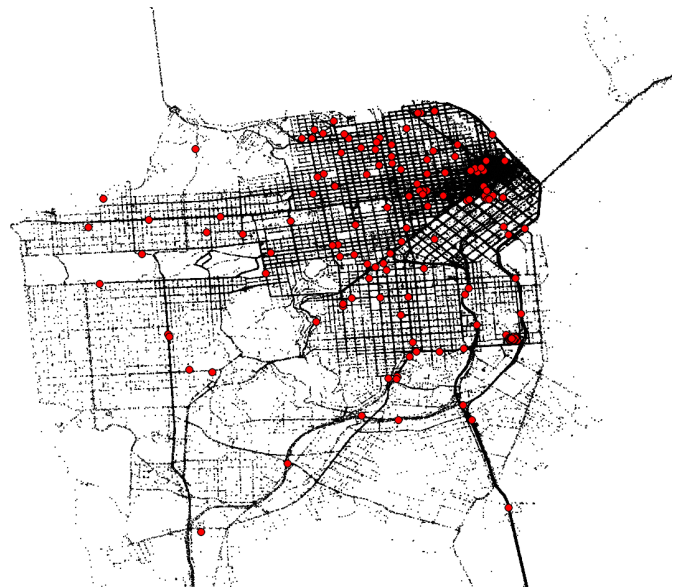
Figure 1. An example of dataset available to Mobile Millennium and processed by the path inference filter: taxicabs in San Francisco from the Cabspotting program [9]. Large circles in red show the position of the taxis at a given time and small dots (in black) show past positions (during the last five hours) of the fleet. The position of each vehicle is observed every minute.
