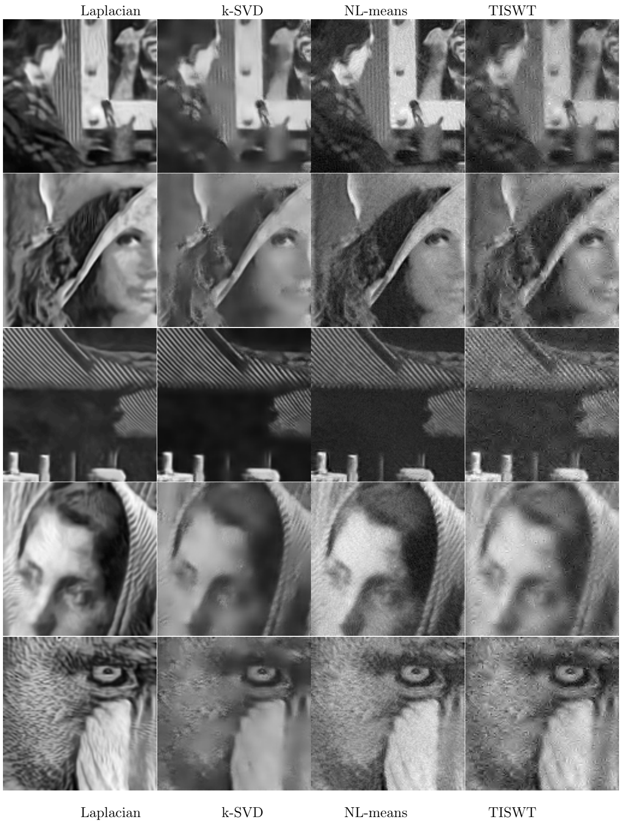
Figure 19: Noise level \sigma = 40 . From left to right: our two-stage approach, k-SVD, nonlocal means, translation-invariant wavelet denoising.
