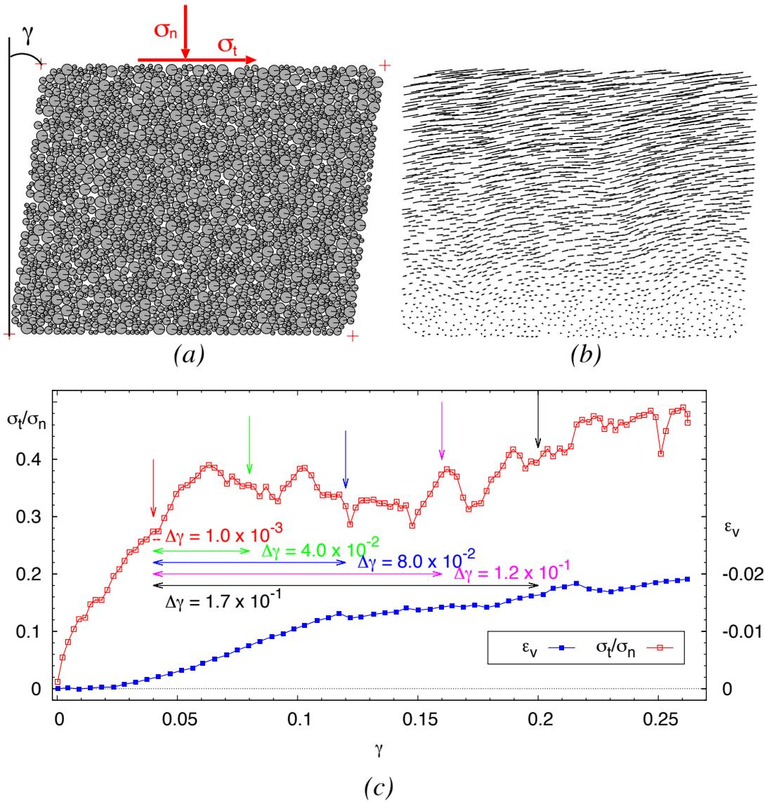
Fig. 2. (a) DIC-based image of granular assembly at  $\gamma = 0.12$ ; (b) displacements of individual grains from  $\gamma = 0$  to  $\gamma = 0.12$  (maximum displacement is approximately 60 mm); (c) stress ratio and volumetric strain ( $\varepsilon_v > 0$  for contraction) as a function of shear strain.
