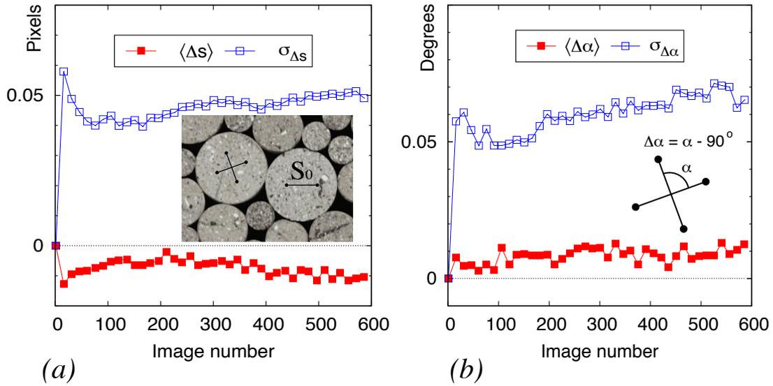
Fig. 3. Accuracy of particle tracking: (a) average (red) and standard deviation (blue) of measured changes of length  $\Delta s$  of 434 segments (initial length 60 pixel); (b) average (red) and standard deviation (blue) of measured changes of angle  $\Delta\alpha$  of 217 pairs of (initially perpendicular) segments.
