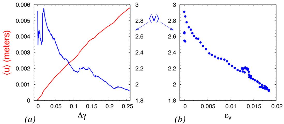
Fig. 4. (a) evolution of the mean values of the norm of fluctuations,  $\langle u \rangle$  and normalized fluctuations,  $\langle V \rangle$  as a function of  $\Delta\gamma$  (at  $\gamma = 0$ ); (b) evolution of  $\langle V \rangle$  with the volumetric strain of the sample.
