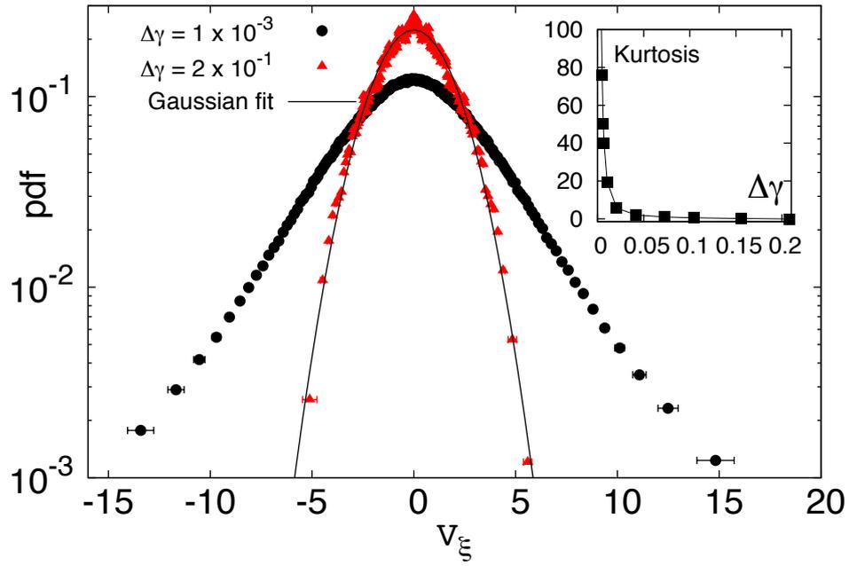
Fig. 5. Probability density function (pdf) of normalized fluctuations  $V_\xi$  projected on the major principal direction  $\xi$  of strain for two different strain windows,  $\Delta\gamma = 10^{-3}$  and  $\Delta\gamma = 2 \times 10^{-1}$ . The major principal direction is given by  $\xi = \tan^{-1}[\gamma/(\epsilon_x - \epsilon_y)]$ . The inset shows the kurtosis of the pdf as a function of  $\Delta\gamma$ .
