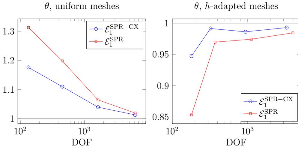
Figure 5: Problem 1.a. Evolution of the effectivity index  $\theta$  considering locally equilibrated,  $\mathcal{E}_1^{\text{SPR-CX}}$ , and non-equilibrated recovery,  $\mathcal{E}_1^{\text{SPR}}$ , for uniform (left) and  $h$ -adapted (right) meshes.
