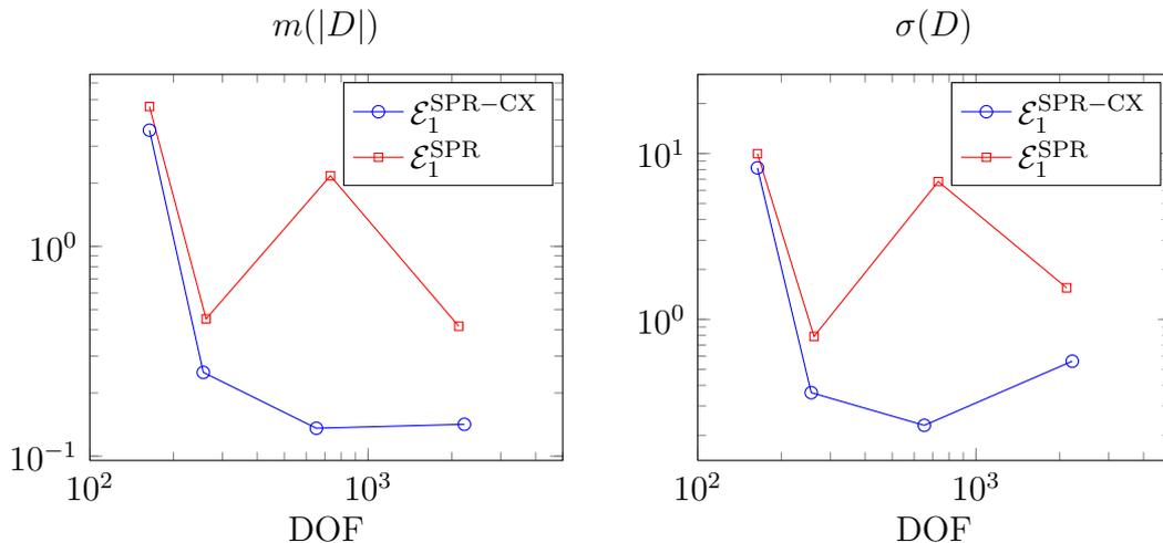
Figure 16: Problem 2. Evolution of the mean absolute value  $m(|D|)$  and standard deviation  $\sigma(D)$  of the local effectivity considering locally equilibrated,  $\mathcal{E}_1^{\text{SPR-CX}}$ , and non-equilibrated recovery,  $\mathcal{E}_1^{\text{SPR}}$ .
