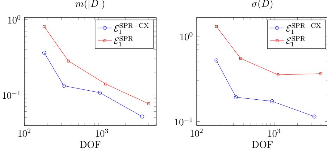
Figure 6: Problem 1.a. Evolution of the mean absolute value  $m(|D|)$  and standard deviation  $\sigma(D)$  of the local effectivity considering locally equilibrated,  $\mathcal{E}_1^{\text{SPR-CX}}$ , and non-equilibrated recovery,  $\mathcal{E}_1^{\text{SPR}}$ .
