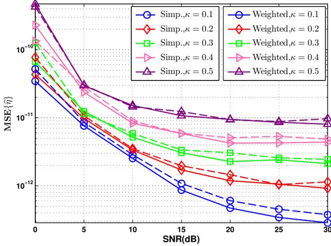
Fig. 6.  $\text{MSE}\{\hat{\eta}\}$  under different accuracy of channel estimation;  $\kappa \in [0.1 : 0.5]$ ,  $M = 10$ ,  $Q = 4$ ,  $\eta = 5 \times 10^{-5}$ ,  $\epsilon = 0.02$ , and  $\text{SNR} \in [0, 30]$  dB.
