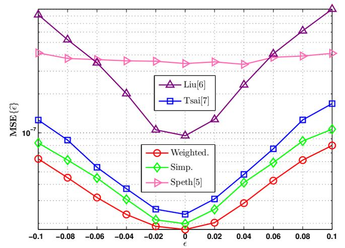
Fig. 5.  $MSE\{\hat{\epsilon}\}$  under different  $\epsilon$ ;  $M = 10, Q = 4, \eta = 5 \times 10^{-5}, \epsilon \in [-0.1 : 0.1]$ , and  $SNR = 20$  dB.
