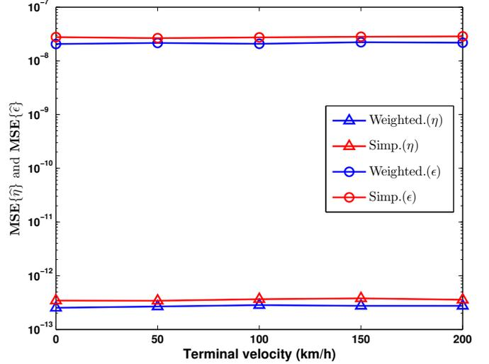
Fig. 7.  $\text{MSE}\{\hat{\eta}\}$  and  $\text{MSE}\{\hat{\epsilon}\}$  under different terminal velocity;  $M = 10$ ,  $Q = 4$ ,  $\eta = 5 \times 10^{-5}$ ,  $\epsilon = 0.02$ , and  $\text{SNR} = 20$  dB.
