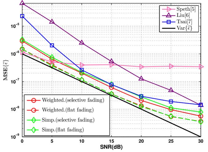
Fig. 3.  $MSE\{\hat{\epsilon}\}$  comparison among different estimators;  $M = 10, Q = 4, \eta = 5 \times 10^{-5}, \epsilon = 0.02$ , and  $SNR \in [0, 30]$  dB.
