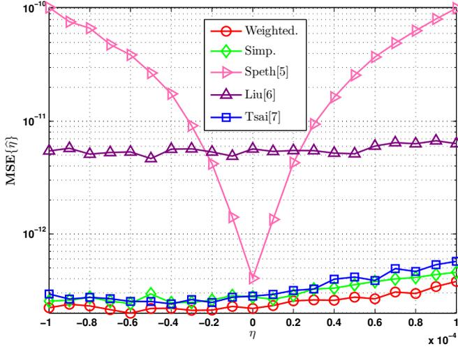
Fig. 4.  $MSE\{\hat{\eta}\}$  under different  $\eta$ ;  $M = 10, Q = 4, \eta \in [-10 : 10] \times 10^{-5}, \epsilon = 0.02$ , and  $SNR = 20$  dB.
