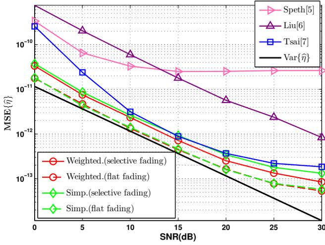
Fig. 2.  $MSE\{\hat{\eta}\}$  comparison among different estimators;  $M = 10, Q = 4, \eta = 5 \times 10^{-5}, \epsilon = 0.02$ , and  $SNR \in [0, 30]$  dB.
