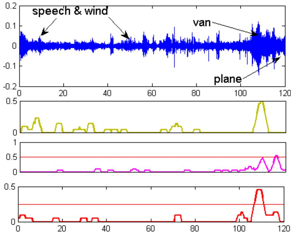
Figure 10.9: Results for test recording #3. The recording contains loud speech during the first 100 seconds, sounds emitted by a car (at around the 105<sup>th</sup> second) and sound of a plane (from the 107<sup>th</sup> second until the end of the recording). The fragment of the first 60 seconds of the recording was part of the training set of the N class.
