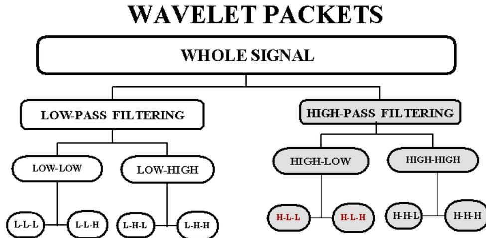
Figure 10.16: Flow of the wavelet packet decomposition.
