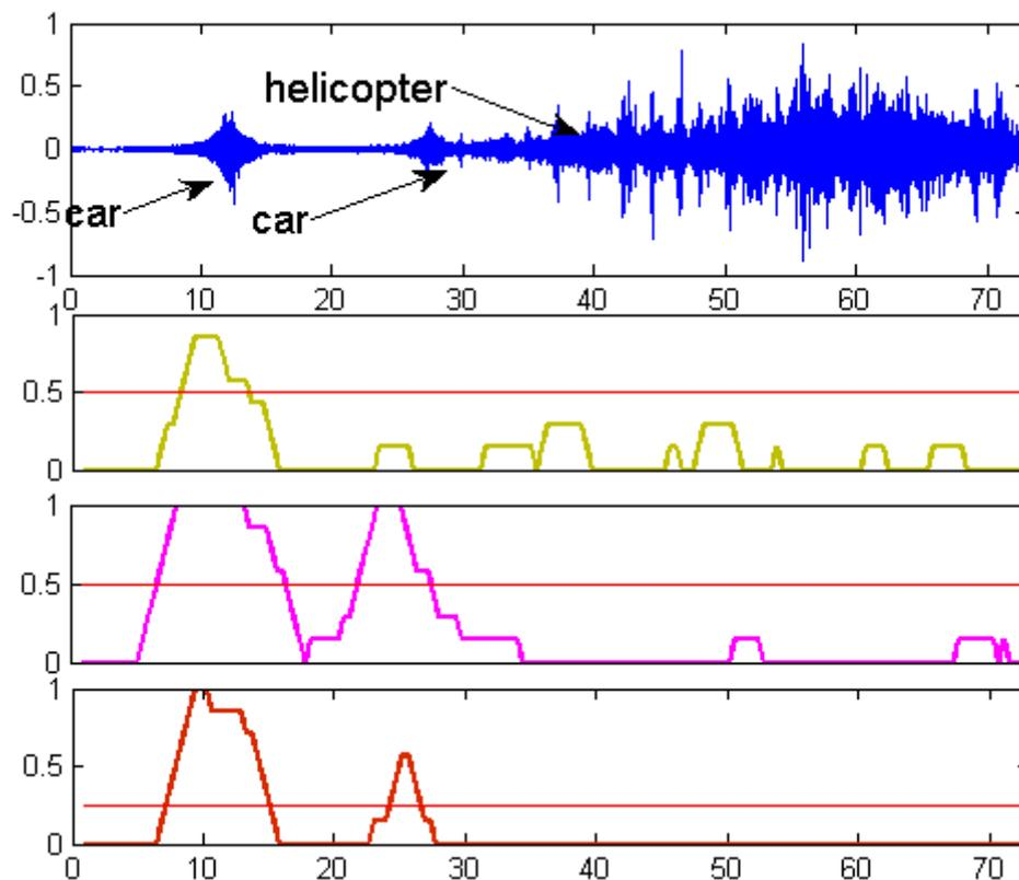
Figure 10.8: Results for test recording #2. The recording contains sounds emitted by a car (at the 11<sup>th</sup> second) and by another car (at the 27<sup>th</sup> second). This recording was part of the training set.
