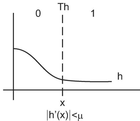
Figure 8.2: An example how to use the histogram  $h$  for finding the threshold value.  $Th$  is set to to the smallest  $x$  for which  $|h'(x)| < \mu$ .
