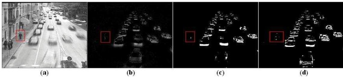
Figure 8.7: (a) The background for the test frame  $s$ . (b) The test frame  $s$  after the subtraction of the background. (c) The output for the test frame  $s$ . (d) The output for the test frame  $s$  from the parallel version of the algorithm.
