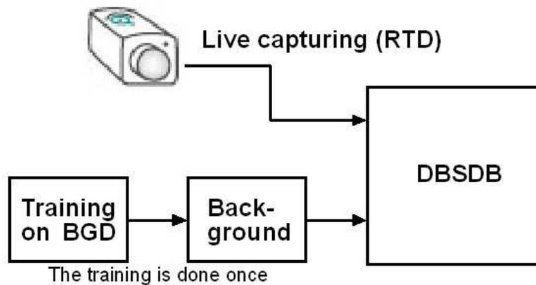
Figure 8.3: The inputs to the DBSDB algorithm. The training is done once on the BGD. It produces the background which is input to the DBSDB. The RTD is the on-line input to the DBSDB.
