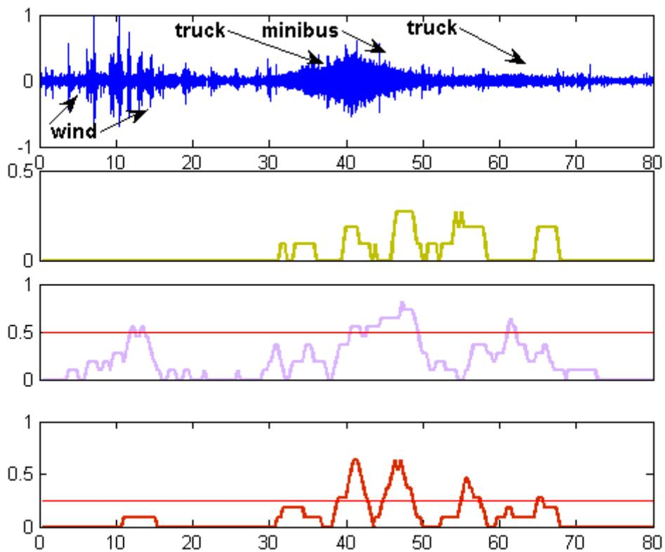
Figure 10.14: Results for test recording #8. A truck followed by a minibus passed by the receiver at around the 40<sup>th</sup> second of the recording. Another truck passed by at around the 65<sup>th</sup> second. Strong wind was present. This recording was not part of the training set.
