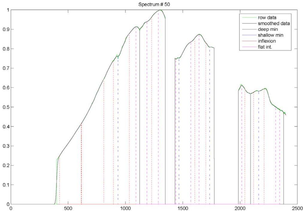
Figure 9.1: Spectrum #50. Green curve – original raw data, black curve – smoothed data after the application of 4<sup>th</sup>-order B-spline to the raw data, black vertical lines – deep minima, blue vertical lines – shallow minima, magenta vertical lines – flat intervals, red vertical lines – inflection points. Obtained using  $T_1 = 0.003$ ,  $T_2 = 0.002$ ,  $T_3 = 0.001$ ,  $T_4 = 0.001$ ,  $T_5 = 0.0005$ .
