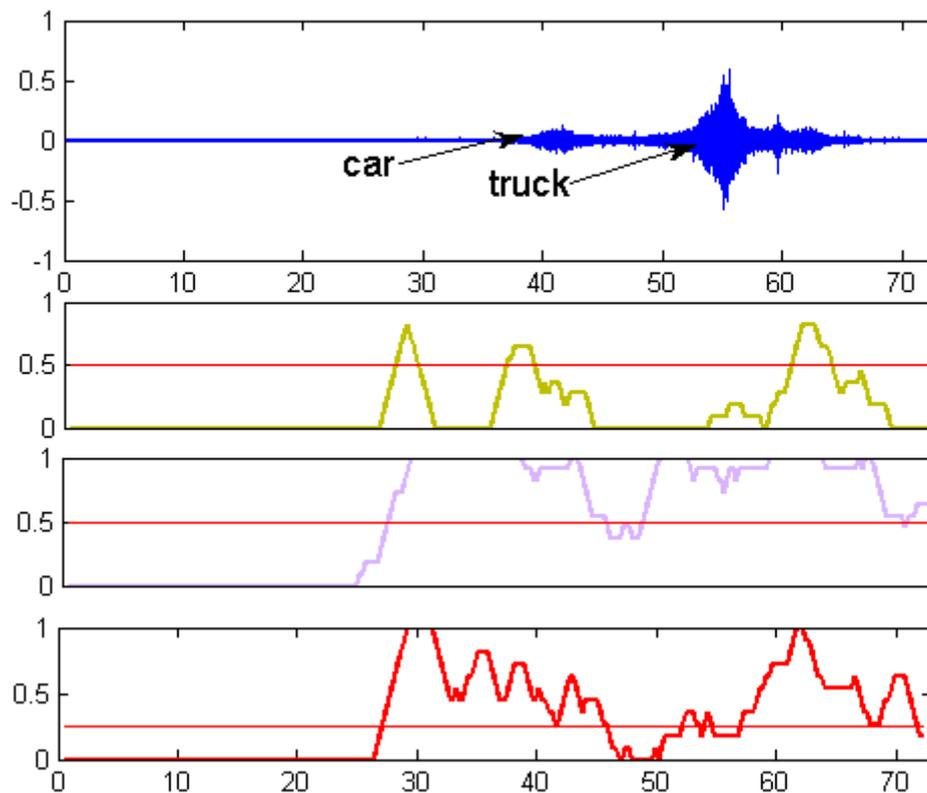
Figure 10.7: Results for test recording #1. The recording contains sounds emitted by a car (at around the 40<sup>th</sup> second) and a truck (at around 55<sup>th</sup> second). This recording was part of the training set.
