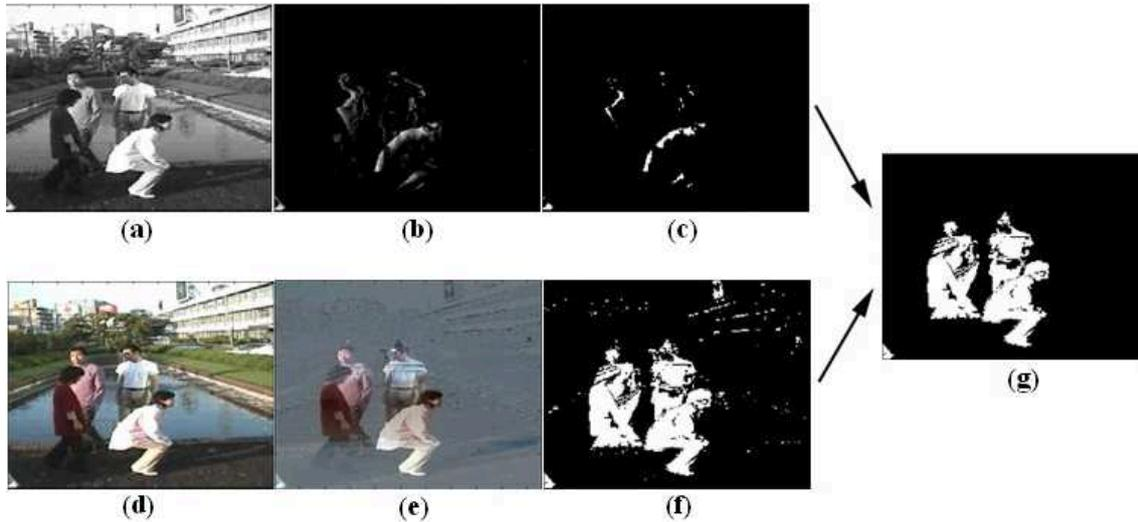
Figure 8.8: (a), (d) The original test frames in grayscale and RGB, respectively. (b), (e) The grayscale and RGB test frames after the background subtraction in the classification steps (steps 3 and 4) of the DBSDB algorithm, respectively. (c), (f) Results after the thresholding of (b) and (e), respectively. (g) The final output of the DBSDB algorithm after the application of the DFS.
