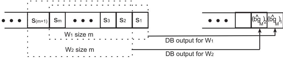
Figure 8.1: Illustration of how the SW is shifted right to left.  $W_1 = (s_1, \dots, s_m)$  is the SW for  $s_1$ .  $W_2 = (s_2, \dots, s_{m+1})$  is the SW for  $s_2$ , etc. The backgrounds of  $s_i$  and  $s_{i+1}$  are denoted by  $(\widehat{bg}_M)_i$  and  $(\widehat{bg}_M)_{i+1}$ ,  $i = 1, \dots, n - m + 1$ , respectively.
