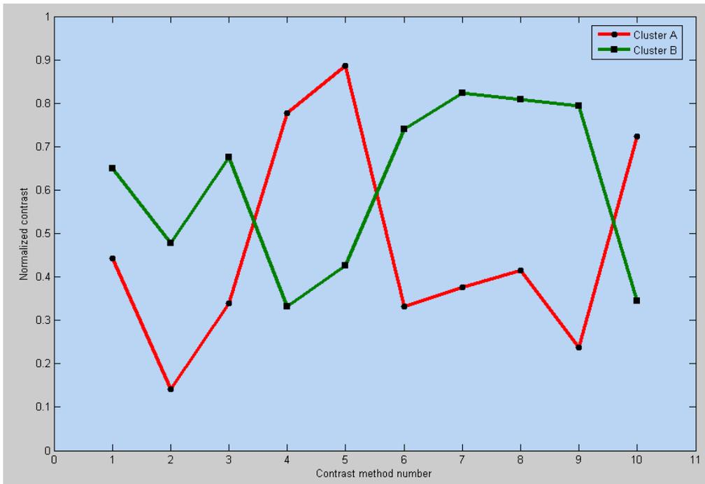
Figure 7.8: Two dissimilar spectra (colored red and green) of two different clusters. The  $x$ -axis depicts the contrast acquisition-method number from Table 7.2 and the  $y$ -axis depicts the values of the spectra for each contrast acquisition-method.
