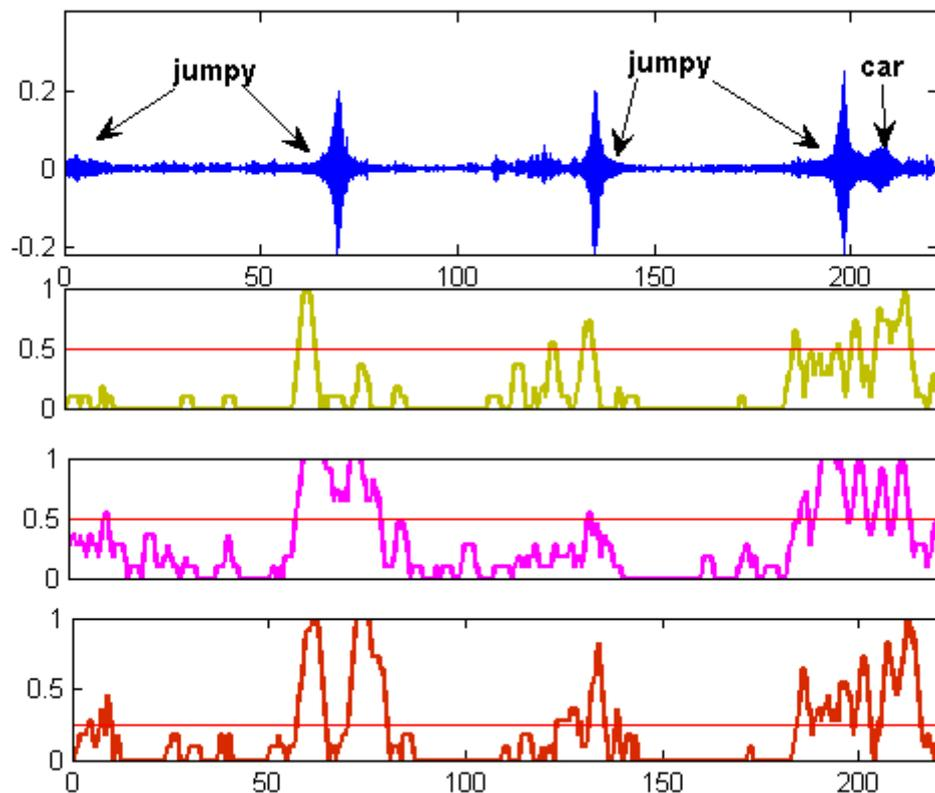
Figure 10.10: Results for test recording #4. In the beginning, the sound from a remote vehicle is heard. A jumping vehicle passed by the receiver at around the 70<sup>th</sup>, 134<sup>th</sup> and 200<sup>th</sup> seconds of the recording. In its last occurrence, it was followed by another car. The recording was not part of the training set.
