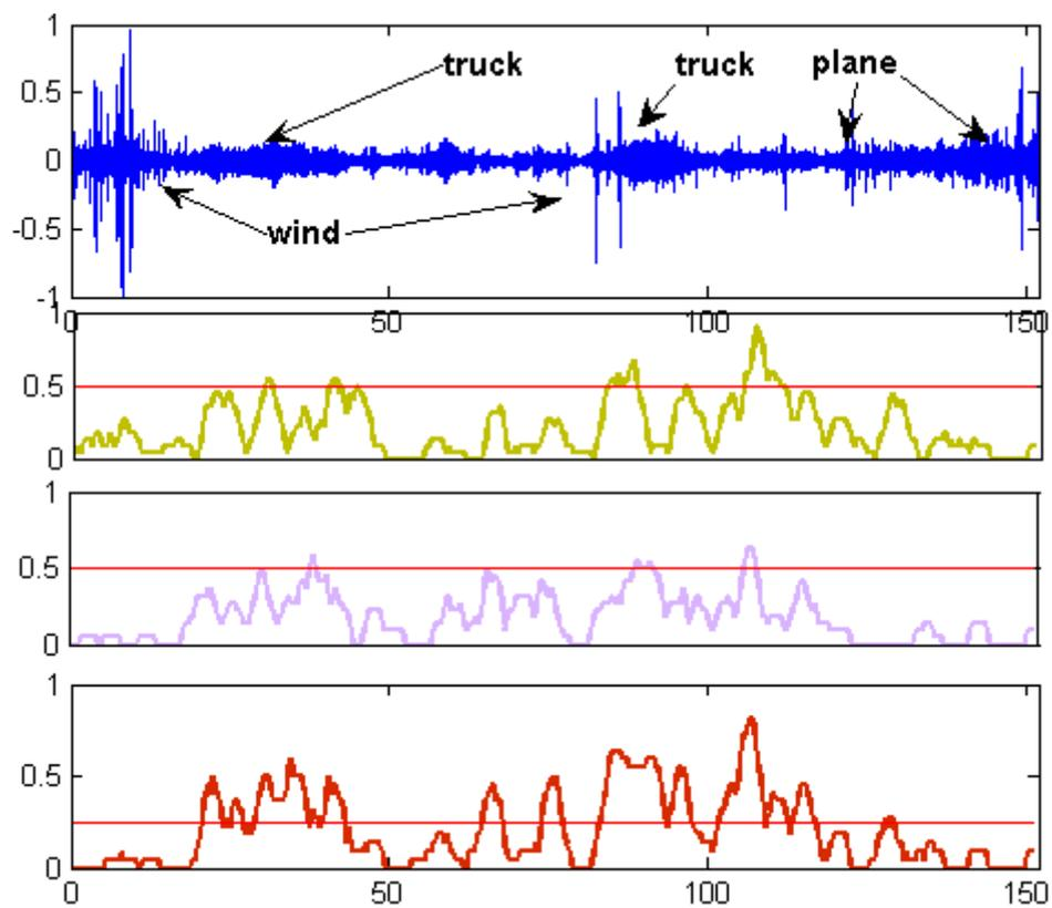
Figure 10.15: Results for test recording #9. A sound of a truck was heard between the 15<sup>th</sup> and the 50<sup>th</sup> seconds and also between the 80<sup>th</sup> and the 110<sup>th</sup> seconds of the recording. An airplane sound appeared next. It lasted until the end of the recording. This recording was not part of the training phase.
