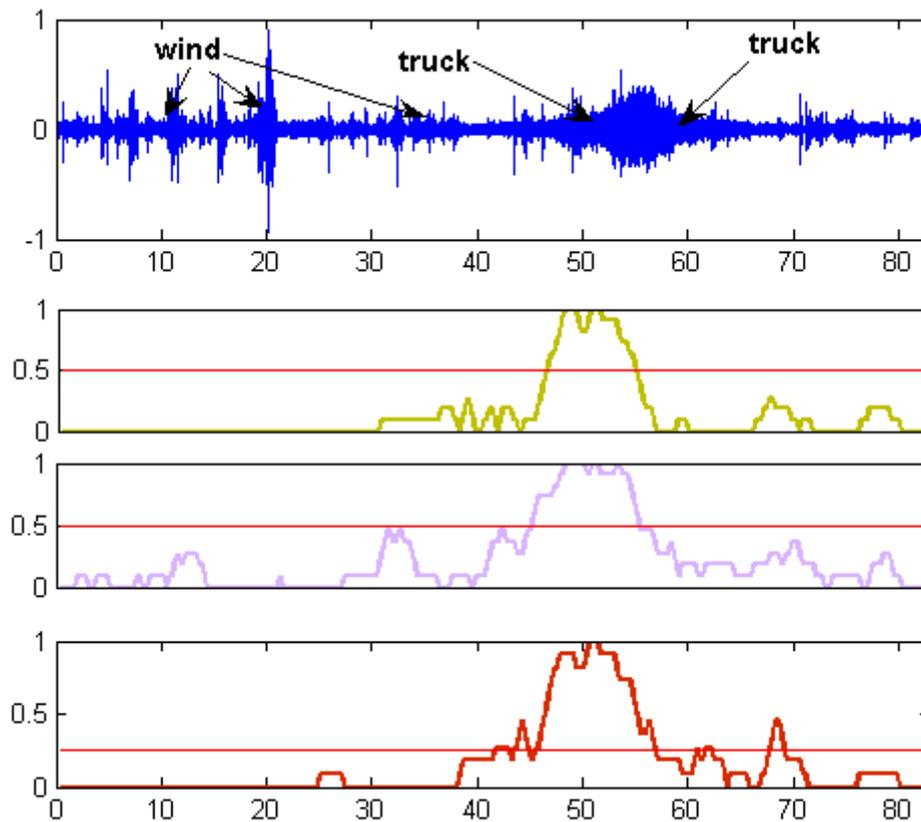
Figure 10.12: Results for test recording #6. Two trucks passed by the receiver in opposite directions at around the 50<sup>th</sup> second of the recording. Strong wind was present at the site. The recording was not part of the training set.
