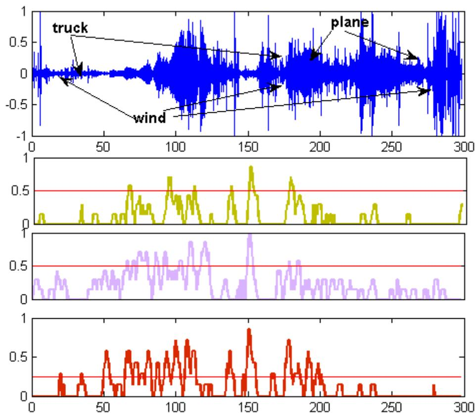
Figure 10.13: Results for test recording #7. A truck passed by the receiver from the 30<sup>th</sup> second to the 190<sup>th</sup> second of the recording. Then, a strong sound of an airplane dominated the recording until the end of the recording. Strong wind sound appeared throughout the recording. This recording was not part of the training set.
