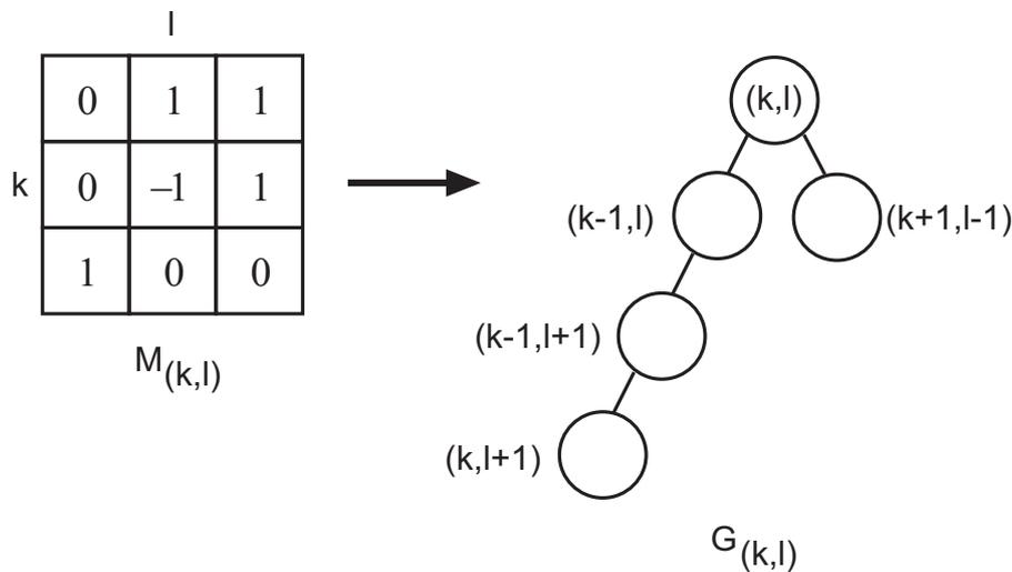
Figure 8.5:  $G_{(k,l)}$  is a graph representation of the 8-neighborhood matrix  $M_{(k,l)}$  whose root is the pixel  $\tilde{s}_i^{rgb}(k, l)$ . A root pixel is set to -1, a foreground pixel is set to 1 and a background pixel is set to 0.
