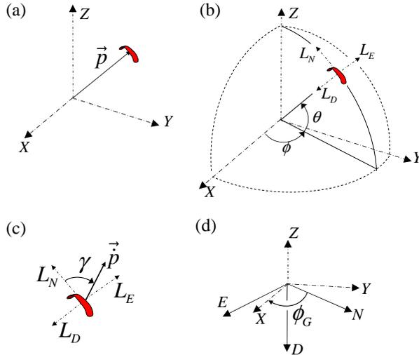
Figure 2: (a) Coordinate system  $G$  and position of the wing  $\vec{p}$ ; (b) local coordinate system  $L$  and spherical coordinates  $\theta$ ,  $\phi$ ; (c) wing velocity angle  $\gamma$ ; (d) coordinate systems  $G$  and  $NED$  and angle  $\phi_G$ .
