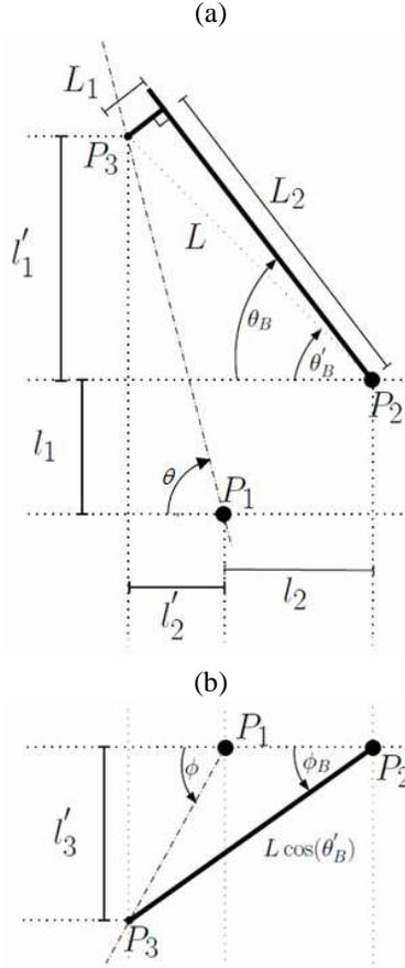
Figure 5: Diagram of the line angle sensor: (a) side view with  $\phi = 0$  and (b) top view. Dash-dotted line: center line of the wing; thick solid lines: metal rod and pulley linking the encoders to the center line.
