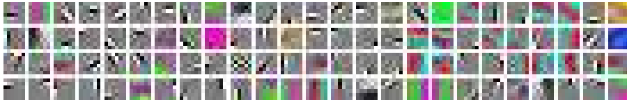
Figure 8: Features learned by a sparse auto-encoder from small image patches
