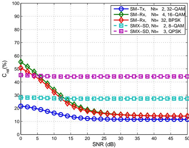
Fig. 8. Computational complexity against SNR.  $m = 6$ , and  $N_r = 4$ .
