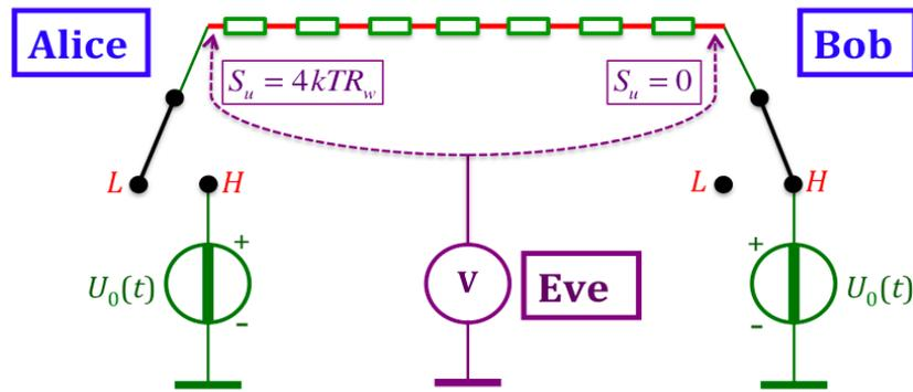
**Figure 7. BR's scheme with finite wire resistance and Johnson noise attack.** With a wire resistance of  $R_w$  and in the steady-state mode, Eve will measure a zero-power density spectrum  $S_u$  at the closed end of the wire and  $S_u = 4kTR_w$  at the open end.
