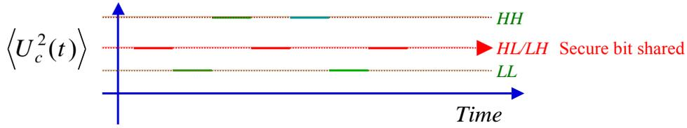
**Figure 2. Mean-square voltage (and current) versus time during operation.** There are three different levels (dotted lines) depending on the actual bit values; the intermediate value indicates a secure bit exchange period.
