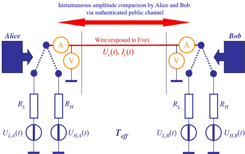
**Figure 3. KLJN system minimally armed against invasive (active) attacks, including the man-in-the-middle-attack.** Alice and Bob measure the instantaneous channel voltage and current amplitudes and compare them via an authenticated public channel. In this way, they learn all the information Eve can have. Additions to prevent hacking—such as line filters, blinding detectors, *etc*—are not shown. The notation is the same as in Fig. 1.
