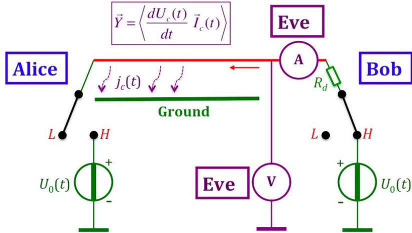
**Figure 6. Transient-damping-resistor version of BR's scheme, and capacitive noise current attack.** The direction and the location-dependent value of the cross-correlation vector  $\vec{Y}$  for the time-derivative of the channel voltage and the current vector provide two ways to crack the key, while the location-dependence of the RMS channel current offers a third way.
