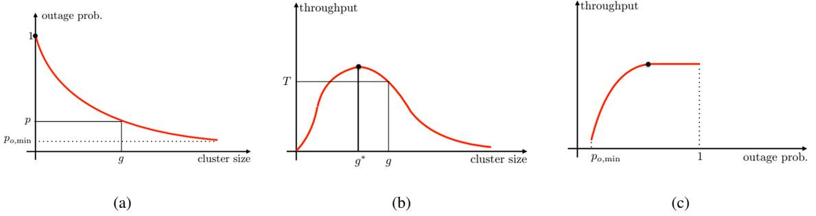
Fig. 3. Qualitative behavior of the tradeoff between throughput and outage probability, by ways of the tradeoff parameter  $g$ , which represents the size of the cluster of nodes over which any node can look for its desired requested file and download it by D2D on-hop communication.
