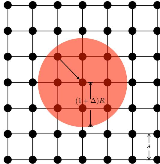
Fig. 2. Grid network with  $n = 49$  nodes (black circles) with minimum separation  $s = \frac{1}{\sqrt{n}}$ . The red area is the disk where the protocol model imposes no other concurrent transmission.  $R$  is the case transmission range and  $\Delta$  is the interference parameter, such that the forbidden disk around the receiver has radius  $(1 + \Delta)R$ .
