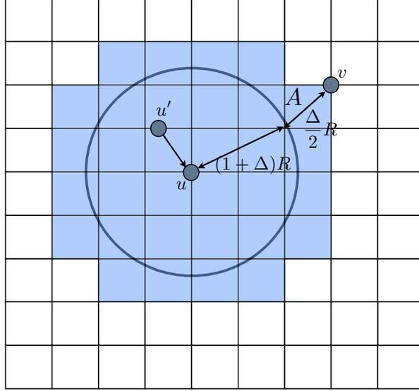
Fig. 7. In this figure,  $u'$  is a transmitter and  $u$  is a receiver.  $v$  is another receiver corresponding to another transmitter. The diagonal of each squarelet is  $\frac{\Delta}{2}R$ . The maximum area that are consumed by receiver  $u$  is the disk centered at  $u$ , with radius  $(1 + \Delta)R$ . The blue squarelets are the maximum activated squarelets that are caused by the active receiver  $u$ .  $A$  indicates the squarelet containing receiver  $v$ .
