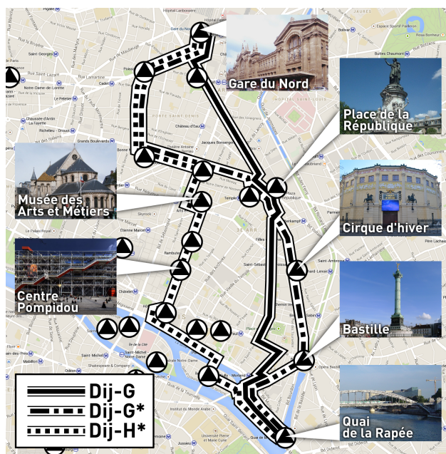
Figure 1: Shortest (continuous) and alternative paths (dot dashed and dotted) alongside PoIs in the city of Paris. This result is an output of the algorithms presented in this paper.
