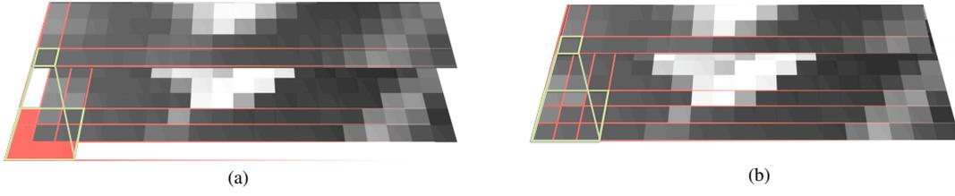
Fig. 1. Illustration of the convolution operators (7) and (8) assuming a blur support of  $3 \times 3$ . a) With the use of (7) we assume that the blurry image  $f$  and the sharp image  $u$  have the same support, therefore we must choose how the values at the boundaries of  $u$  are defined (red pixels); b) With (8) we assume that  $f$  has a smaller support than  $u$ , therefore the pixels of  $f$  are completely defined by the pixels of  $u$ .
