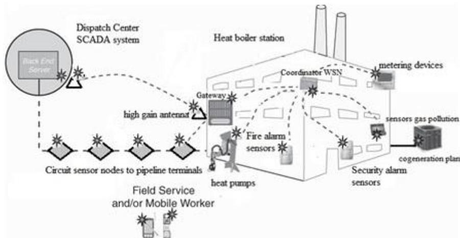
Fig. 1. - Sensor network cluster for heating points
