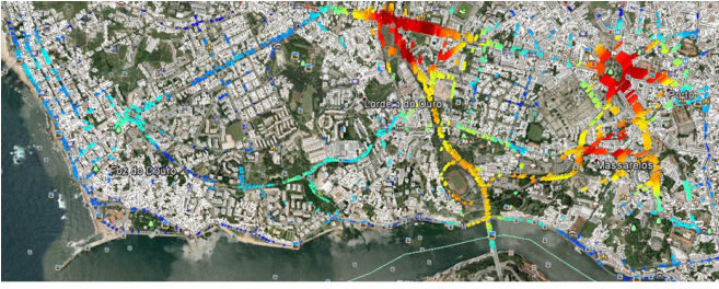
Fig. 15. Urban environment (Porto, Portugal) used for simulations. The map overlay shows the number of directly reachable vehicles (“neighbors”) for each vehicle, as generated by the GEMV^2 model. For each vehicle, the colored bar represents the number of neighbors. Warmer and taller bar colors indicate more neighbors.
