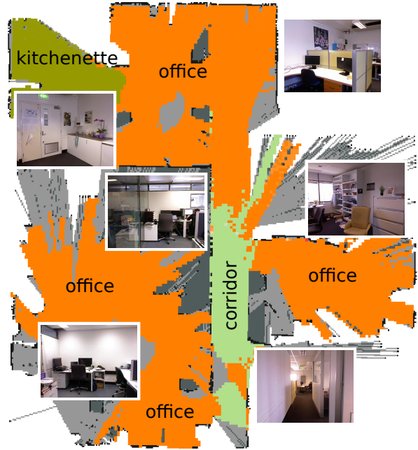
Fig. 1: A semantic map generated by the system described in this paper. The colors encode the semantic categories of different places encountered in the environment. The figure shows a map of an office environment (orange) with a kitchenette (dark green) and a long corridor (light green).
