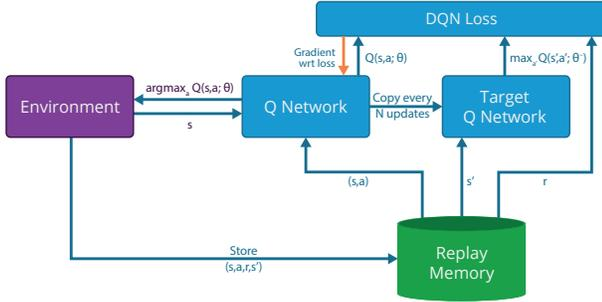
Figure 1. The DQN algorithm is composed of three main components, the Q-network ( $Q(s, a; \theta)$ ) that defines the behavior policy, the target Q-network ( $Q(s, a; \theta^-)$ ) that is used to generate target Q values for the DQN loss term and the replay memory that the agent uses to sample random transitions for training the Q-network.
