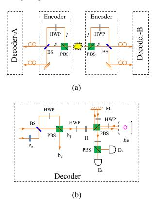
FIG. 5: (Color online) Schematic setup for entanglement distribution.  $p_{\pi}$  is a  $\pi$  phase shifter.
