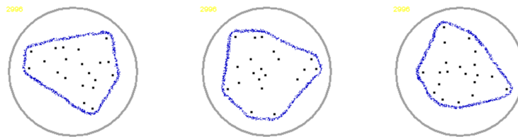
Fig. 22. Convex Hull via shrinkage around hazard stimuli. Three separate examples are shown. A band of model plasmodium shrinks around the set of points to approximate the Convex Hull. Note a small peripheral region is indicated because of the repulsive region.
