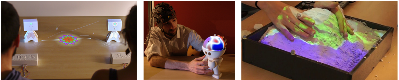
Figure 1: (Left) Tobe is a toolkit enabling the creation of tangible augmented customized bio- and neurofeedback. Here, two users are relaxing together by using Tobe to reach cardiac coherence. (Middle) Teegi is an augmented tangible avatar that displays the user's brain activity in real time. (Right) Inner Garden is an augmented sandbox, linked to the user's inner states via physiological sensors, designed for contemplative play.
