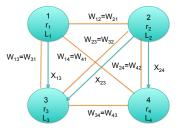
Figure 2. A network flow model of the robust taxi dispatch problem. A circle represents a region with region ID 1, 2, 3, 4. We omit the superscript of time k since every parameter is for one time slot only. Uncertain demand is denoted by  $r_i$ ,  $L_i$  is the original number of vacant taxis before dispatch at region i, and  $X_{ij}$  is a dispatch solution that sending the number of vacant taxis from region i to region j with the distance  $W_{ij}$ .
