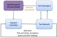
Figure 1. A prototype of the taxi dispatch system
