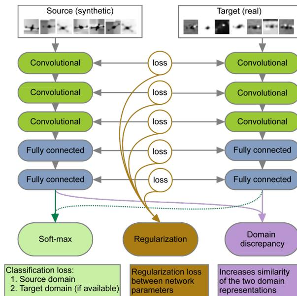
Figure 1. **Our two-stream architecture.** One stream operates on the source data and the other on the target data. Their weights are *not* shared. Instead, we introduce loss functions that prevent corresponding weights from being too different from each other.
