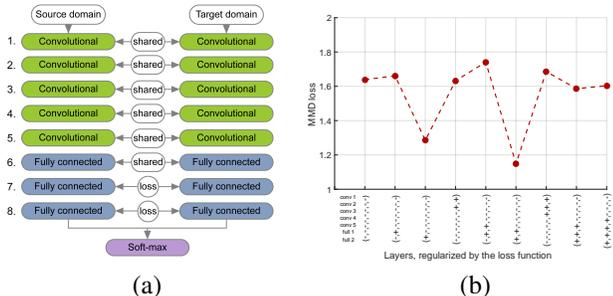
Figure 6. Office dataset. (a) The network architecture that proved to be the best according to our MMD-based criterion. (b) The  $y$ -axis corresponds to the  $MMD^2$  loss between the outputs of the corresponding streams that operate on *Amazon* and *Webcam*, respectively. The  $x$ -axis describes the configuration, as in Fig. 3.
