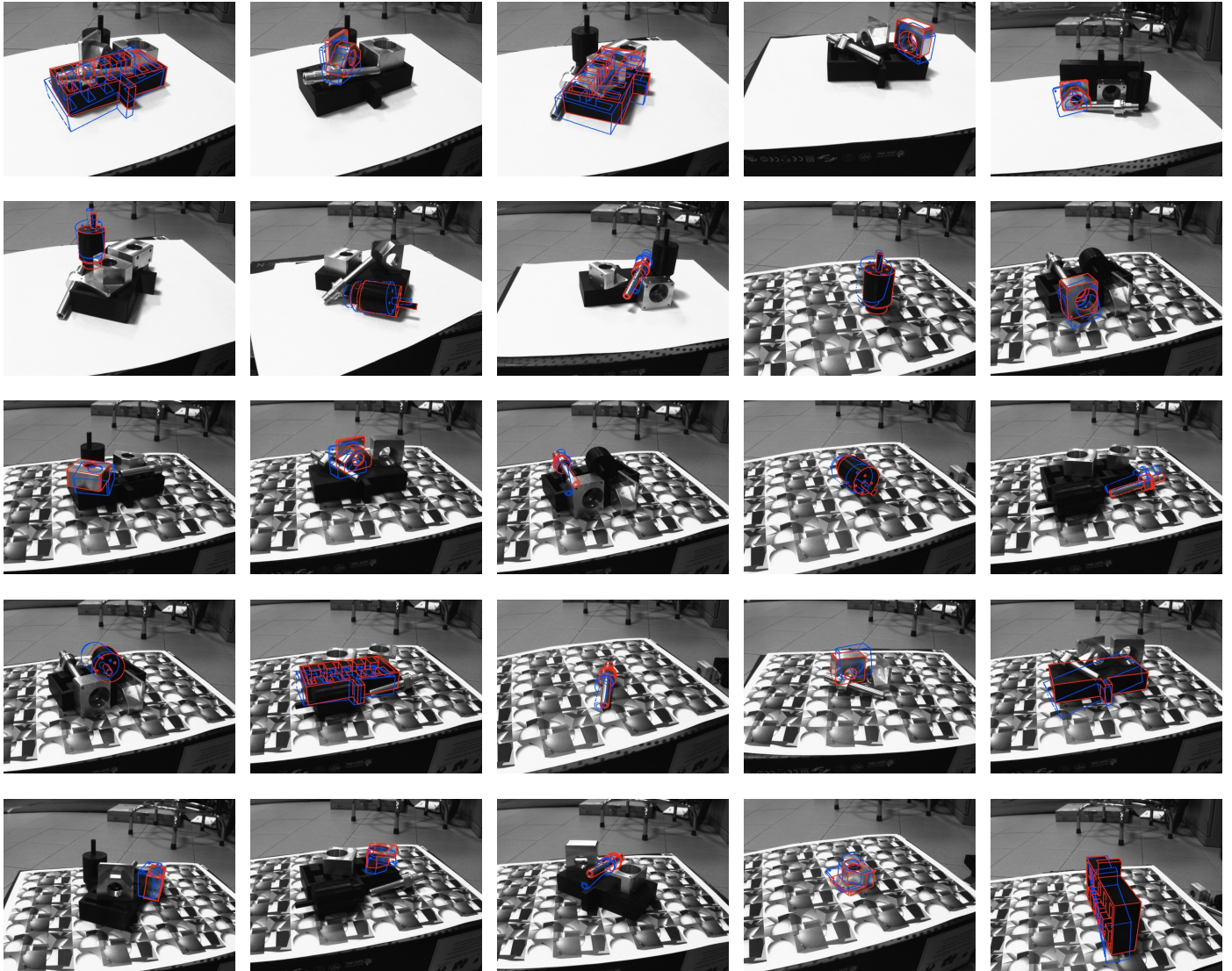
Figure 11: Some registration results obtained using the single-view D 2 CO algorithm ( Dataset 1 ), the initial guess is reported in blue, while the final position estimate is reported in red.
