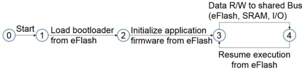
Fig. 8. State machine of the MCU of a generic IoT.
