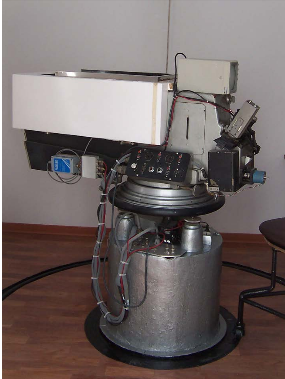
Figure 5. Modified Danjon astrolabe (courtesy of the ROA archive).
