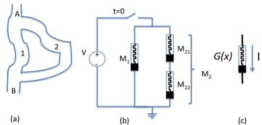
Fig. 1. (a) Points A (nest) and point B (food source) are connected through two paths L1 and L2, such that  $L2=2L1$ . (b) Memristive network model of the ant colony model in (a).
