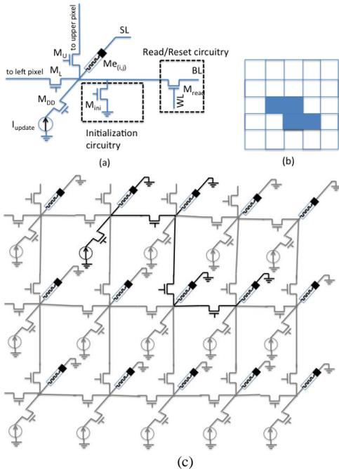
Fig. 10. (a) Implementation of each pixel for voltage based memristive devices. (b) A sample pattern of ant traversal. (c) Illustration of connections of adjacent pixels for voltage based memristive devices.
