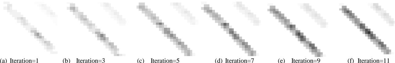
Fig. 5. The amount of pheromone deposited on the pixel map of Fig. 3 (a) as the ant colony algorithm progresses.
