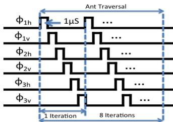
Fig. 15. Timing diagram of the control signals for ant traversal.
