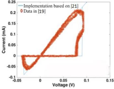
Fig. 12. Comparison of the implementation of model in [21] with the experimental data in [19].
