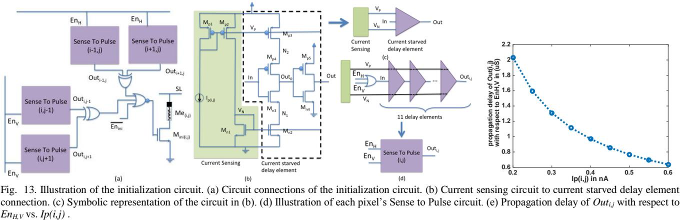
Fig. 13. Illustration of the initialization circuit. (a) Circuit connections of the initialization circuit. (b) Current sensing circuit to current starved delay element connection. (c) Symbolic representation of the circuit in (b). (d) Illustration of each pixel's Sense to Pulse circuit. (e) Propagation delay of  $Out_{i,j}$  with respect to  $En_{H,V}$  vs.  $Ip(i,j)$ .
