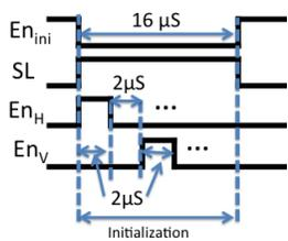
Fig. 14. Timing diagram of the control signals for initialization.
