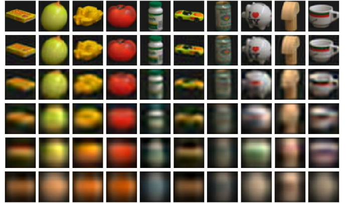
Fig. 3. The reconstruction of Coil-100 dataset by using TRSVD. The top row shows the original images, while the reconstructed images are shown from the second to sixth rows corresponding to \epsilon=0.1, 0.2, 0.3, 0.4, 0.5 , respectively.
