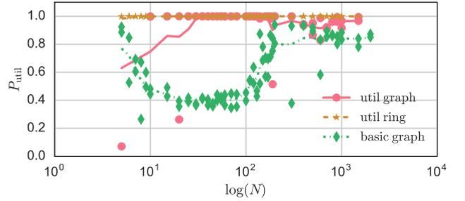
Fig. 5. Power utilization for step pricing and agents with utility function described in this section. The green line shows the utilization for the basic model.
