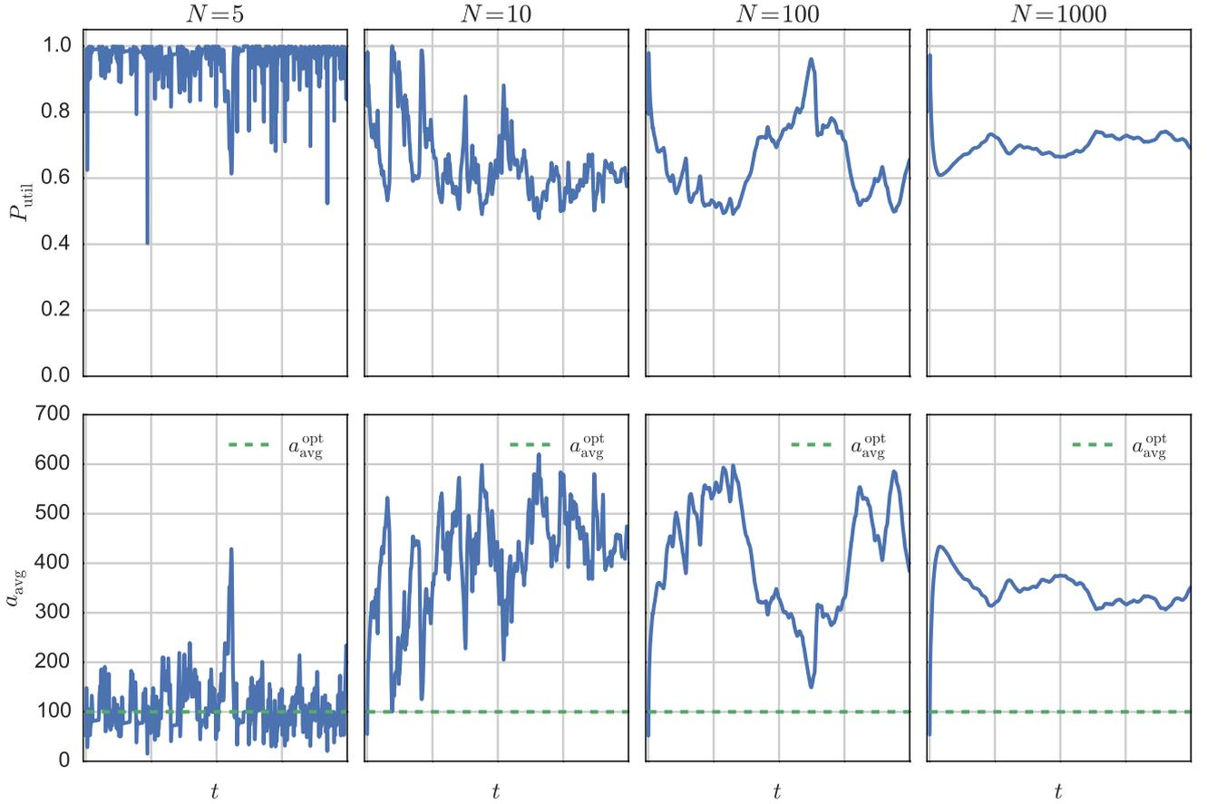
Fig. 3. Typical behavior of very small ( $N = 5$ ), small ( $N = 10$ ), medium ( $N = 100$ ) and large systems ( $N = 1000$ ). The small systems can operate much closer to the optimum, while mid-size systems show big jumps after stable periods. The system parameters are  $\lambda_{\min} = 0.005$ ,  $R_V = 2\Omega$ ,  $R_0 = R/N = 200\Omega$ ,  $p_{\text{err}} = 0.01$  and  $V = 1\text{V}$ . The communication network is configured as a ring.
