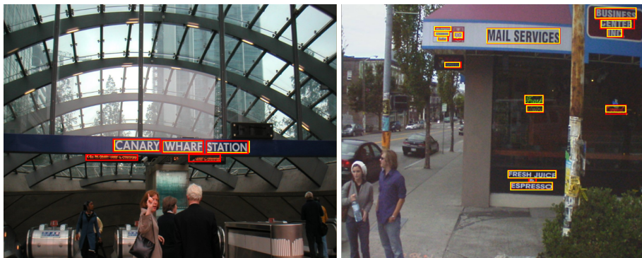
Fig. 6: CTPN detection results on extremely small-scale cases (in red boxes), where some ground truth boxes are missed. Yellow boxes are the ground truth.
