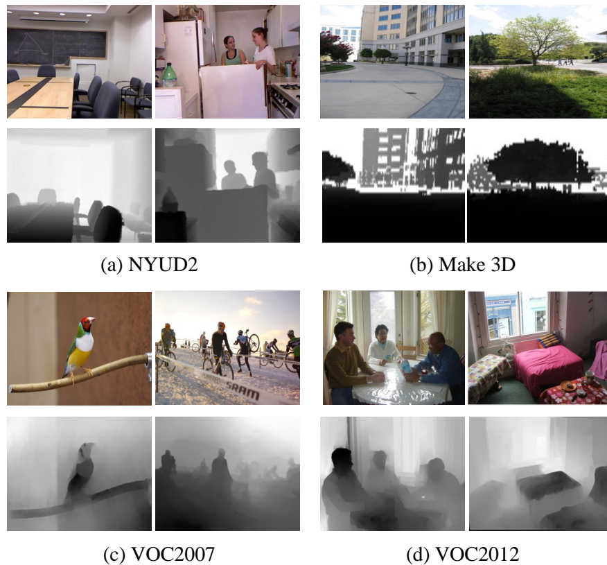
Fig. 1: Examples of ground-truth depth maps and estimated depth maps. (a) NYUD2 dataset (ground-truth) (b) Make3D dataset (ground-truth) (c) VOC2007 dataset (estimated) (d) VOC2012 dataset (estimated).
