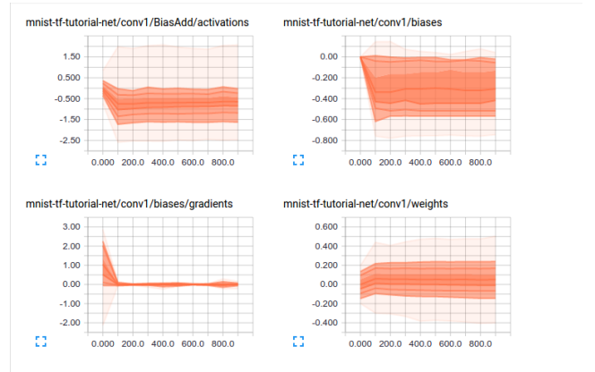
Figure 5: Visualization of how distribution of multi-dimensional tensors change over time. Each line on the chart represents a percentile in the distribution over the data: for example, the bottom line shows how the minimum value has changed over time, and the line in the middle shows how the median has changed. Reading from top to bottom, the lines have the following meaning: [maximum, 93%, 84%, 69%, 50%, 31%, 16%, 7%, minimum] These percentiles can also be viewed as standard deviation boundaries on a normal distribution: [maximum, \mu+1.5\sigma , \mu+\sigma , \mu+0.5\sigma , \mu , \mu-0.5\sigma , \mu-\sigma , \mu-1.5\sigma , minimum] so that the colored regions, read from inside to outside, have widths [ \sigma , 2\sigma , 3\sigma ] respectively.
