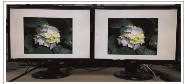
Figure 4. Demonstration of implemented invisible embedded data for smart digital signage system. (Right side display contains an original video image while the left one includes the embedded data inside the image of the video).
