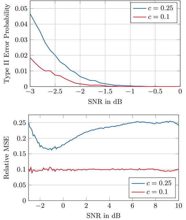
**Fig. 2:** Detection and estimation performance of the proposed algorithm for  $\alpha = \beta(\theta) = 0.05$  and  $c \in \{0.1, 0.25\}$ .
