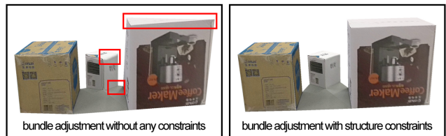
Figure 8. A comparison of results obtained using Bundle adjustment without structure constraints and with structure constraints.
