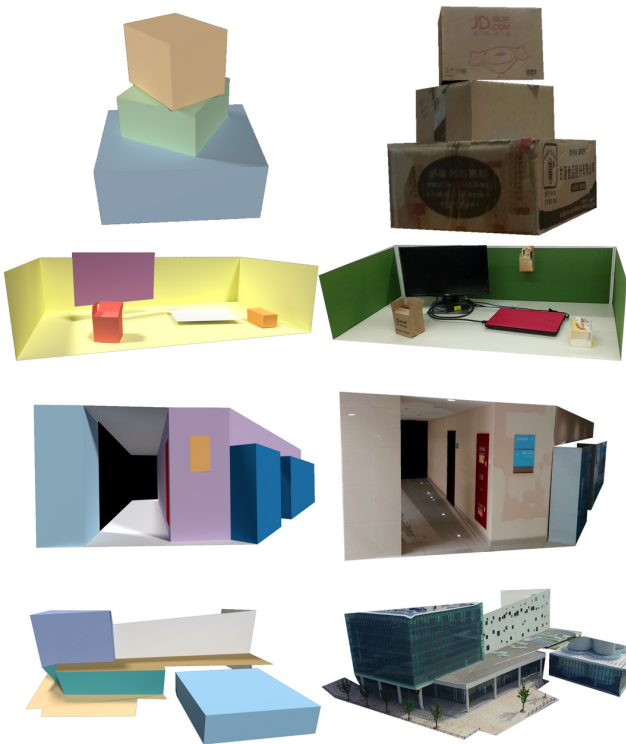
Figure 10. 3D models (color shaded and textured) obtained using our algorithm on data set in Figure 9. Our method faithfully recovers both the plane geometry and plane arrangements.
