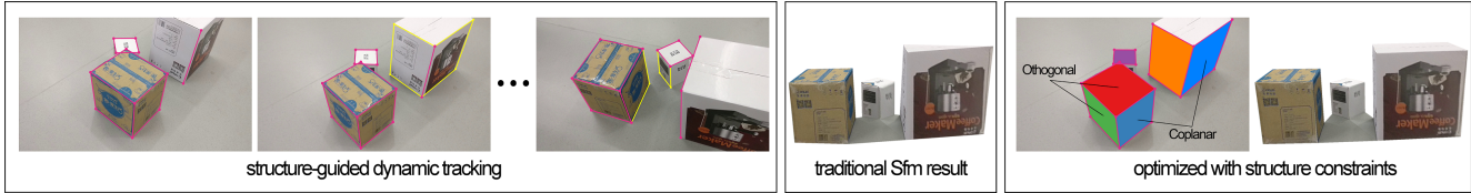
Figure 2. The pipeline of our method. Given the initial marked frame, our method first propagates the structure points across the rest frames by a structure-guided dynamic tracking algorithm, followed with a relation-augmented joint optimization which simultaneously solves for the plane geometry and the plane-to-plane inter-relations (arrangements). Yellow lines are newly added edges which do not appear in previous frames.
