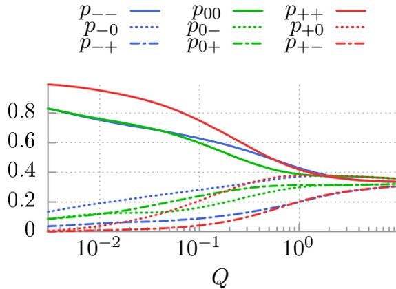
FIG. 5. All transition probabilities between the three observed states: the minus  $v_- = -0.4$ , the zero  $v_0 = 0$  and the plus  $v_+ = 0.4$  solution. In the regime  $Q = 0.0045$  corresponding to the maximal diffusion coefficient there are significant differences between them which disappear as temperature is increased. Other parameters are the same as in Fig. 2.
