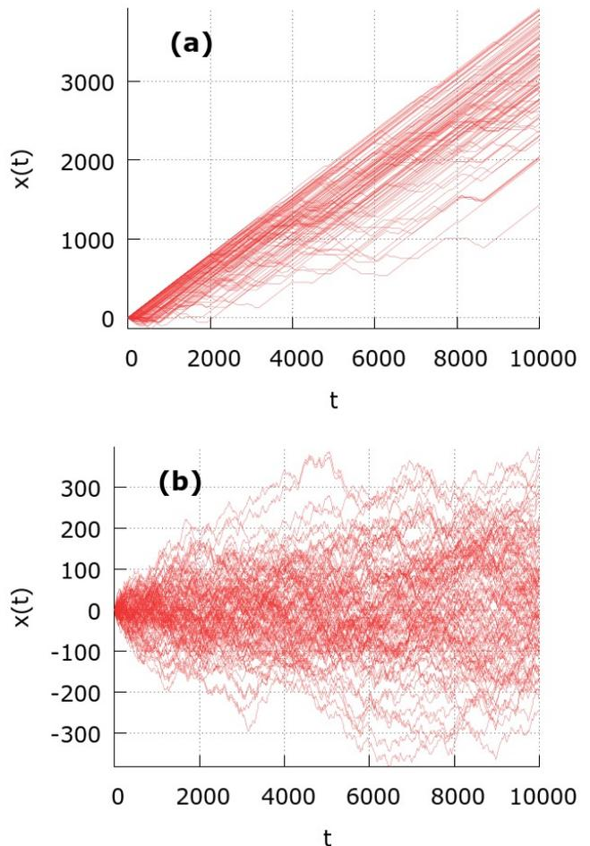
FIG. 7. Typical sample trajectories of the Brownian particle coordinate  $x(t)$  are depicted for different temperature of the system  $Q = 0.0045$  (panel (a)) and  $Q = 0.76$  (panel (b)). In panel (a) transition between the states  $v_- = -0.4$ ,  $v_0 = 0$  and  $v_+ = +0.4$  are clearly visible. The long lasting periods of motion corresponding to the zero  $v_0$  and the minus  $v_-$  solutions lead to enlargement of the diffusion coefficient.
