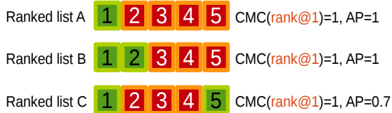
Figure 6: The difference between Average Precision (AP) and CMC measurements. The green and red boxes represent the position of true and false matches in rank lists. For all three rank lists, CMC curve at rank 1 remains 1 whilst AP=1 (rank list A), 1 (rank list B), and 0.7 (list C), respectively.
