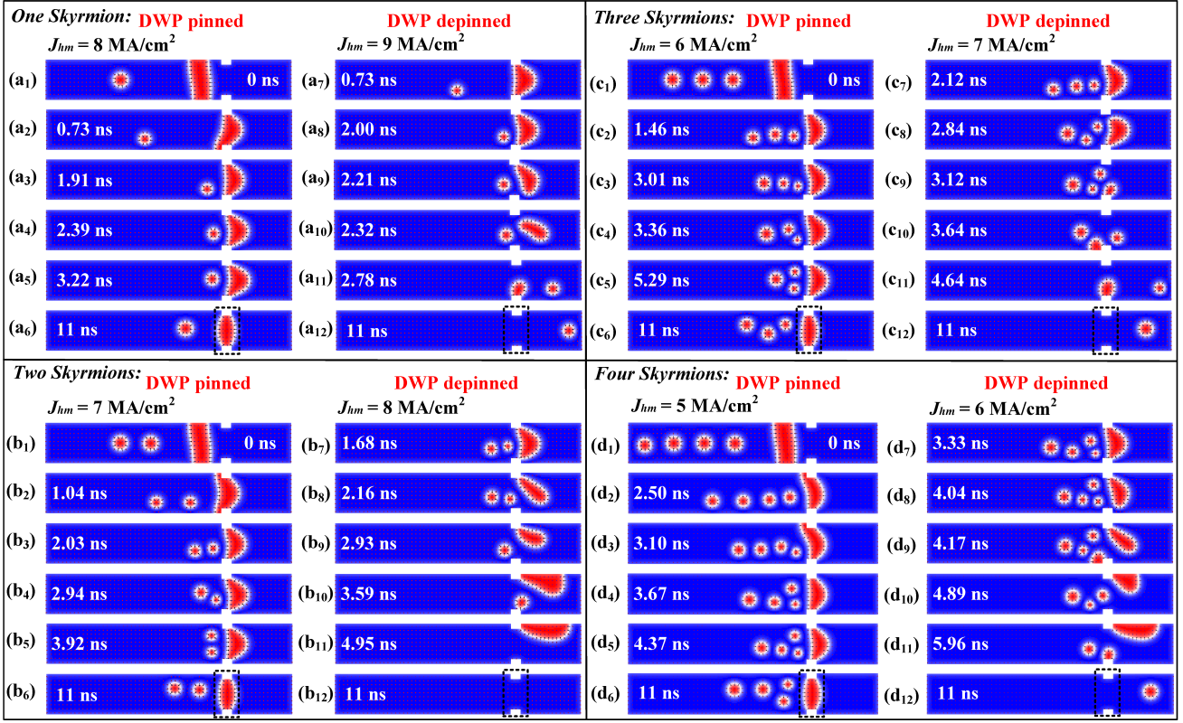
Fig. 2. Micromagnetic simulation result of dynamic interactions between domain wall pair and skyrmion under 10-ns current pulse, with various number of skyrmions and current densities ( J_{hm} ). For the specific number of skyrmions in the nanotrack, increasing the current density can release the domain wall pair from the pinning site.
